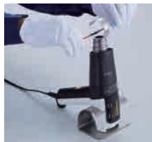
Heat shrink tubing Use of hook type nozzle and stand
